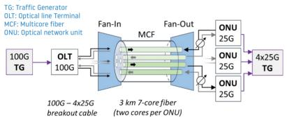
Compared to conventional PON – fronthaul solutions, space division multiplexing - PON (SDM- PON) offers high capacity without complex multiple – input multiple – output digital signal processing (DSP). At mmWave/sub-THz frequencies, the key challenge for implementing fronthaul is how to provide high throughput for each single user. Our results demonstrate that it is possible to achieve nearly optimal performance while keeping the simplicity of non-coherent fronthaul transmission.
