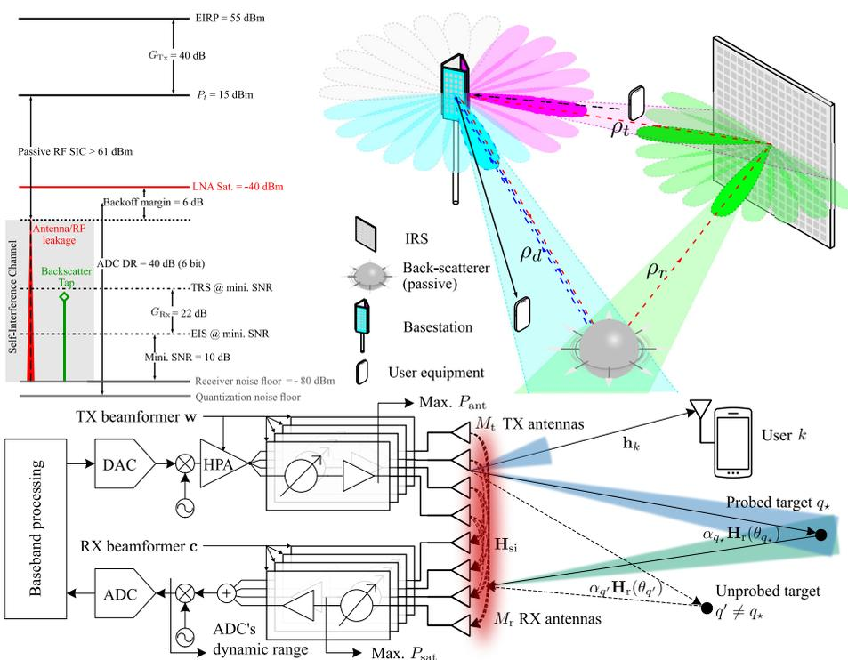
*Strong self-interference poses problems for integrated sensing and communication along the full signal path, like saturation and desensitization. Intelligent reflecting surfaces can be deployed to alleviate these by creating benign additional echo paths. Alternatively, analog beamforming can be designed to satisfy sensing and communication constraints while canceling the self-interference loop.*
