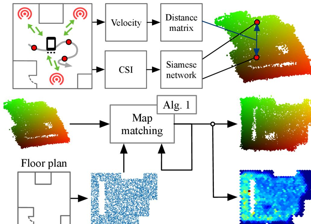
Stage 1 (Top) generates a channel chart based on CSI and velocity information. After the channel chart is generated, it only reflects the radio geometry up to isometries. To exploit the channel chart for localization stage 2 (Bottom) learns a linear transformation to the real-world coordinates by provided topological map information.
