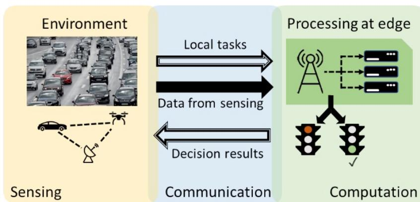
*In future 6G networks, the focus is shifted from data to information. A typical application scenario is to make real-time decisions in a dynamic environment based on certain observations. Such tasks can no longer be fulfilled with sole data communications. Instead, it requires integrating sensing, communication and computation functionalities into the same system and operates cooperatively.*
